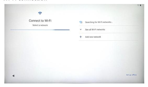
Select an available Wi-Fi network or add one manually. You may setup the device offline, however, it is recommended to connect Thomson Go Plus to the Wi-Fi network for better experience and latest features from Google.
