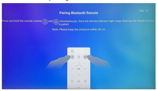
The usage of the remote control can be possible only via Bluetooth. To pair your remote control with Thomson Go Plus, please press & hold the source and the settings buttons simultaneously as shown in the picture or on the Smart Display keeping the distance within 20 cm. After 3
